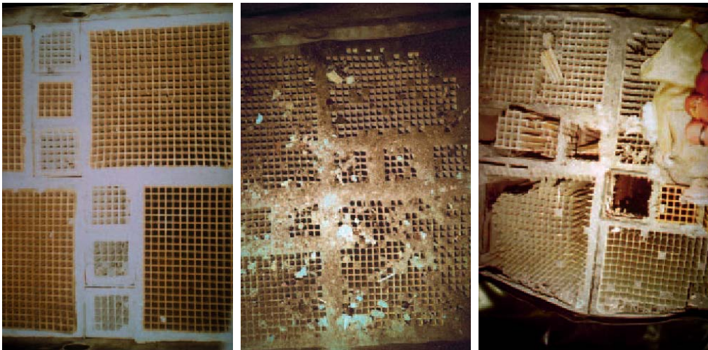
Fig. 3.21. The evolution process in the deterioration of catalyst
